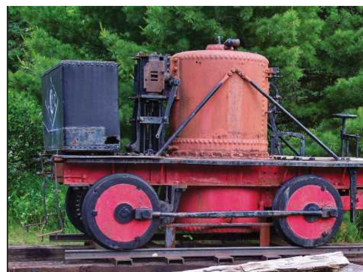
PRIOR TO RENOVATION , the Yankee on display on the Michigan Iron Industry Museum grounds. The Yankee is thought to be one of only three surviving Chaplin locomotives in the world. The Yankee is made from cast and wrought iron, steel and a mix of soft and hardwoods. It is just over 12 feet long, about 9 feet high. The locomotive had been amateurly restored in the late 1930s by employees of the Cleveland-Cliffs Iron Co. and exhibited outdoors, near the company offices, until being donated to the Michigan Iron Industry Museum in 1986.
